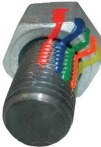
Figure 34: Bolt with 5 Different Torque Stripes
